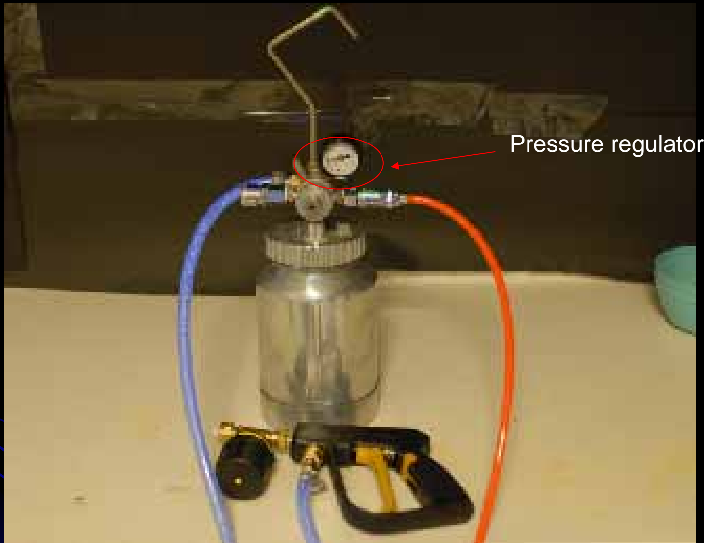
MeterJet Spray Gun Connected to a Pressure Tank
